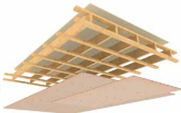
Two layers 13mm GIB X-Block®
