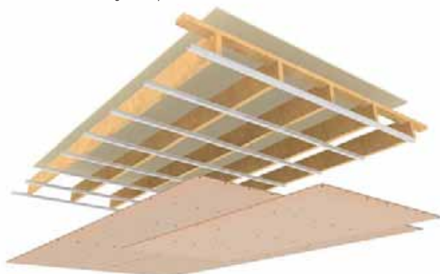
Two layers 13mm GIB X-Block®
